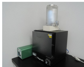
Electric Furnace and Afterburner Device
